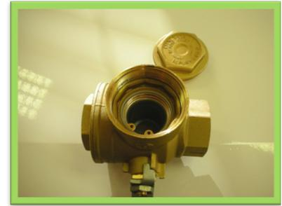
05. Place small pliers into the two bronze holes in the circular clip and pinch together to remove.
