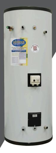
Attractive in appearance with superb heat loss characteristics, Advance Heat Pump Cylinders are supplied with tted T&P valve, immersion heater for thermal disinfection, dual thermostat with control and high limit plus full G3 kit.
